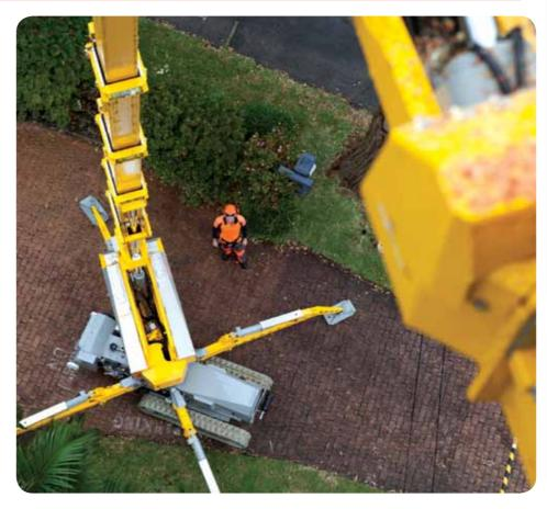
If you are looking for a safer option than climbing on jobs that have risks such as power lines, bark inclusion or visible bracket fungi, then this is the machine for you. With its working height of 37m and a maximum horizontal outreach of nearly 14m, this machine is highly versatile for many applications.
